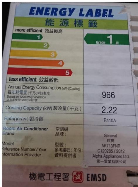
According to the energy label of an air conditioner, the determination of annual energy consumption is based on a 1200 hours/year operation.
