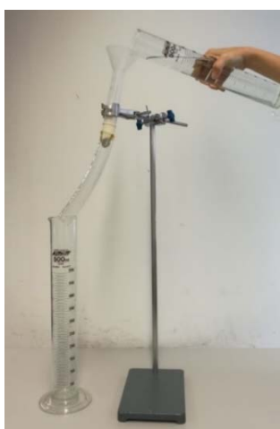
Figure j A set-up for measuring the flow rate of water through the model of aorta with artificial heart valve.
