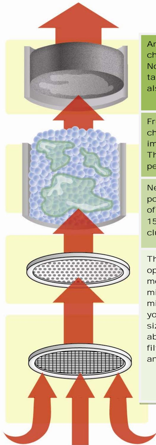
And finally, the water passes through a chamber of granulated active carbon. Not only does the carbon improve the taste and smell of the water, it should also filter out any remaining parasites
