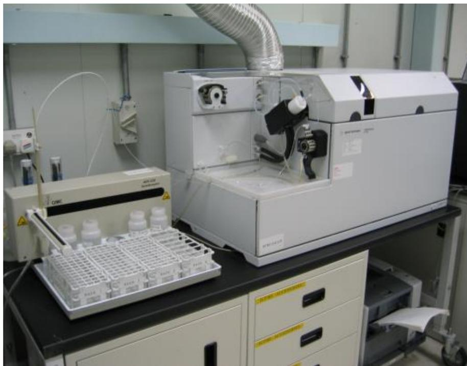
Inductively Coupled Plasma Mass Spectrometer (ICP-MS)
