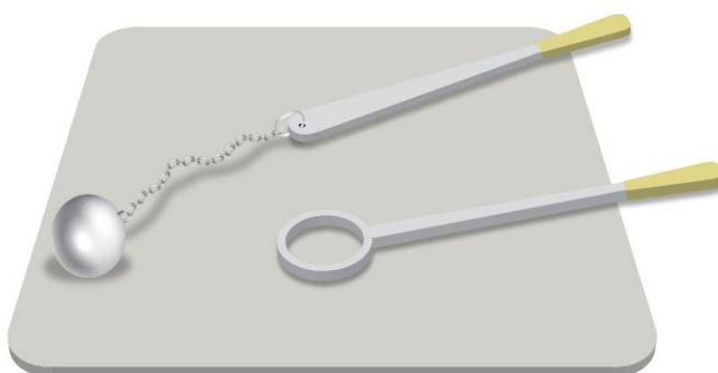
Metal ball and ring are placed on a fireproof mat after heating
