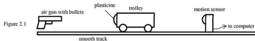
Describe the procedures of the experiment. State the physical quantities to be measured and an equation for finding the speed of the bullet. Write down **ONE** precaution for getting a more accurate result. (5 marks)
