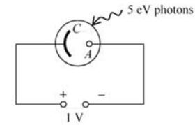
A photocell is connected to a 1 V d.c. source as shown. A monochromatic light beam with each photon of energy 5 eV is incident on cathode C of the photocell so that photoelectrons are emitted. If the work function of cathode C is 2 eV, what is the maximum kinetic energy of the photoelectrons reaching anode A ?
