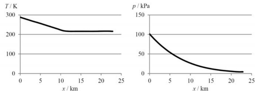
The weather balloon is released and rises to the upper atmosphere. Assume that the temperature and pressure of the helium gas in the balloon are the same as those of the air outside at any height  $x$ .
