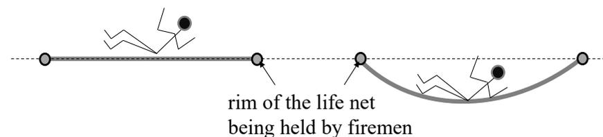
When a person hits the net, it deforms and puts the person to a stop in a longer time as compared to hitting the solid ground.
