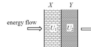
A wall is composed of layers X and Y of U-values  $U_1$  and  $U_2$  respectively. Both layers have the same thickness and dimensions, and there is no air gap between them. Which expression gives the U-value of the wall ?
