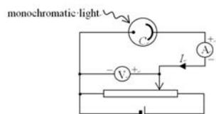
Monochromatic light of fixed intensity is shone on the cathode C of a photocell. The p.d. Applied across the photocell is adjusted and the corresponding current  $I$  is measured. What will be the graph of  $I$  against  $V$ ?
