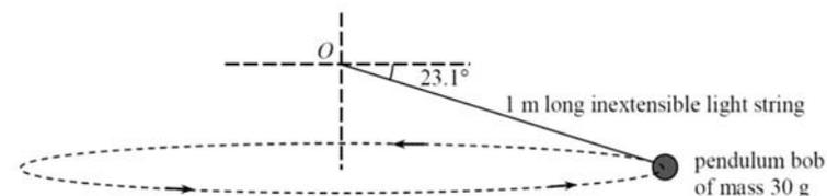
A pendulum bob of mass 30 g is tied to a fixed point  $O$  by a 1 m long inextensible light string. It is swirled to describe a horizontal circle uniformly at an angular velocity of  $5.0 \text{ rad s}^{-1}$  as shown in Figure 4.1. Neglect air resistance. ( $g = 9.81 \text{ m s}^{-2}$ )
