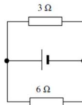
In the above circuit, the cell has e.m.f. 12 V and internal resistance 2 Ω. What is the current in the 6 Ω resistor ?
