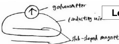
There are 2 factors that can affect the ~~amt~~ induced in a conductor when it moves in a magnetic field. Which are the no. of coils in the magnetic field and the speed of moving the conducting wire. Firstly, connect the conducting wire to the light-beam galvanometer, then place a loop of the conducting wire between the 2 magnets on steel yoke. Move the coil the ~~up~~ up and down and there will be induced current and the light-beam on the galvanometer will move.
