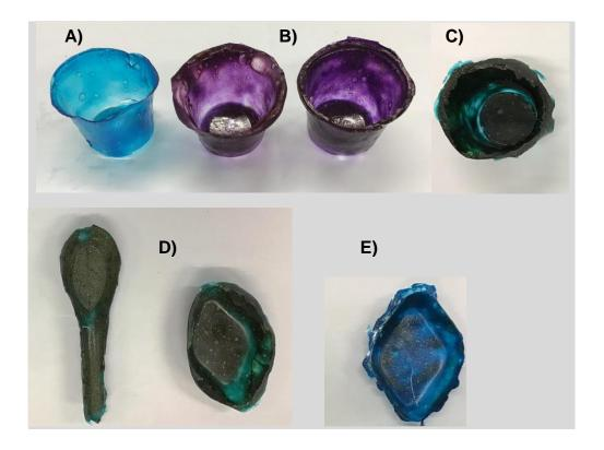
Figure 3.1.2 Bioplastic utensil product models synthesized with different acetic acid concentrations and added with food coloring [A) Chitosan/starch% 50/50, B) Chitosan/cassava flour % 50/50, C) and D) Chitosan/Starch % 25/75, E) Chitosan/cassava flour % 70/30]
