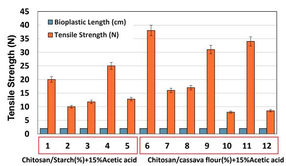
Figure 3.2.1 Tensile strength of synthesized bioplastic 2.0 with different concentration of acetic acid
