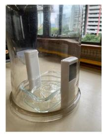
Fig. 2.2 Measurement setup for formaldehyde
