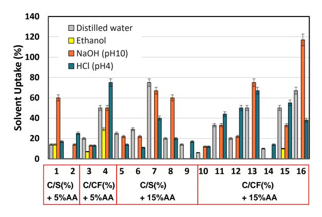
Figure 3.3.1 Solvent absorption capacity of synthesized bioplastic films with different concentration of acetic acid [Key: Chitosan (C); Starch (S); Cassava flour (CF); Acetic acid (AA)]
