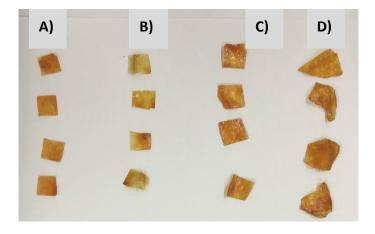
Figure 3.4.1 Bioplastic film samples before biodegradation test [% starch/chitosan; [A) 50/50, B) 60/40, C) 70/30, D) 40/60]
