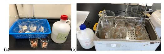
Figure 2.1a Demineralization setup and 2.1b Deacetylation setup
