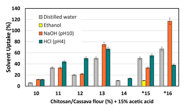
Figure 3.3.A Solvent absorption capacity of synthesized bioplastic with different concentration of acetic acid
