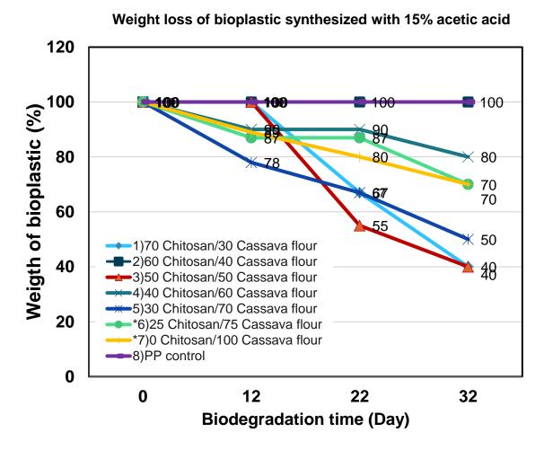
Figure 3.4.2 Biodegradation test of synthesized bioplastic films with different concentration of acetic acid
