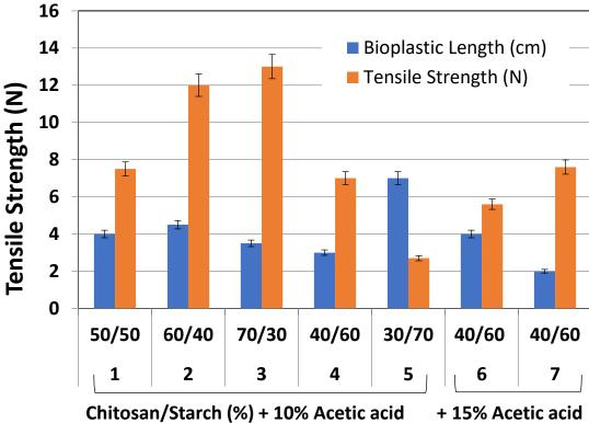
Figure 3.2.A Tensile strength of bioplastic 1.0 with different concentration of acetic acid
