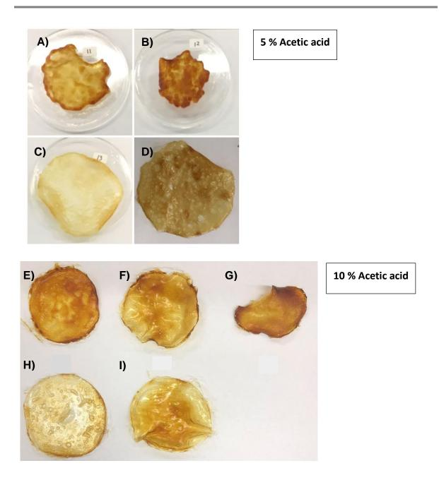
Figure 3.1.1A Bioplastic synthesized with 5% acetic acid [Chitosan/Starch % A) 70/30, C) 30/70; Chitosan/Cassava Flour % B) 70/30, D) 30/70]; Bioplastics synthesized with 10% acetic acid [Chitosan/starch % E) 50/50, F) 60/40, G) 70/30, H) 40/60, I) 30/70].
