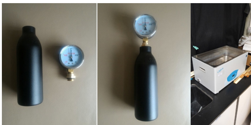
Figures: (left to right) Metal can for pressurised gas, the pressure gauge and heat bath.
